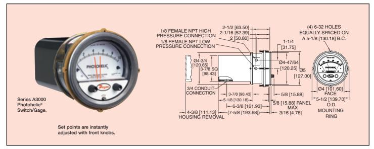
Photohelic® Switch/Gages function as versatile, highly repeatable pressure switches combined with a precise pressure gage employing the time-proven Magnehelic® design. The Photohelic® measures and controls positive, negative or differential pressures of air and compatible gases. Standard models are rated to 25 psig (1.7 bar) with options to 35 (2.4) or 80 (5.5 bar) psig. Single pressure 36000S models measure to 6000 psig (413 bar) with a 9000 psig (620 bar) rating.
