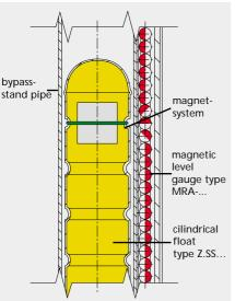
visually. Small plastic or aluminum rollers with inlaid bar magnets are held in an aluminum or stainless steel profile bar. Depending on the level of filling in the stand pipe, these rollers turn from white to red as the level rises and from red to white as the level drops. The filling level inside the vessel can thus be indicated continually without requiring any outside power source.
