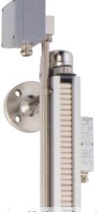
Level sensors are used as pickups for continuous remote electrical indication of the filling level. The magnetic field of the permanent magnet in the cylindrical float acts through the wall to activate very small reed contacts that continually register the measurement voltage on a resistance measurement chain. This measurement voltage is proportional to the filling level (a 3-conductor potentiometer circuit). The resolution of the reed contacts is produced with spa-
