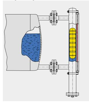
Magnetic level gauges are used for displaying the filling level
